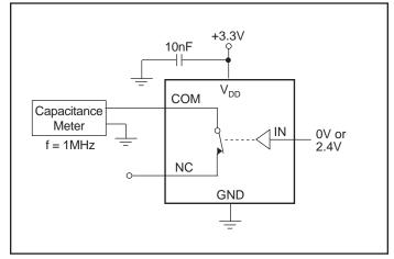
Figure 7. Channel-On Capacitance
