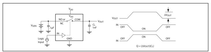
Figure 2. Charge Injection
