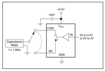
Figure 6. Channel-Off Capacitance
