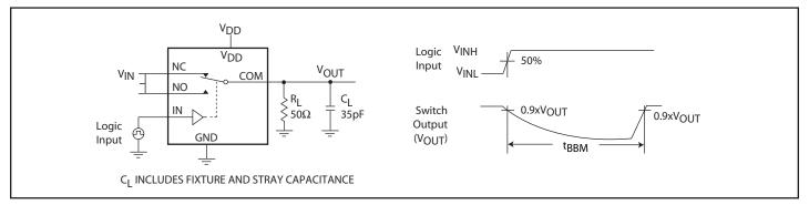
Figure 3. Break-Before-Make Interval
