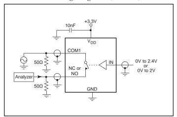
Figure 4. Off Isolation/On-Channel Bandwidth
